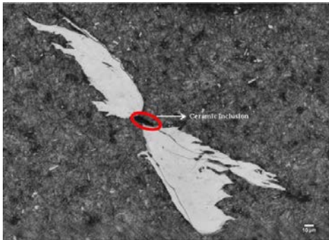
Fig. 2a- Typical 2D optical micrograph of butterfly and initiating inclusion.
