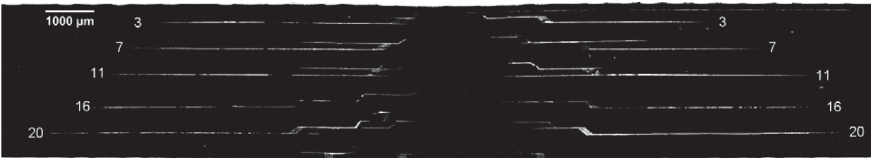
FIGURE 9. Threshold image from the serial sectioning data, highlighting the delamination and matrix crack substructure contained within the serial sectioning volume for specimen D3-5.
