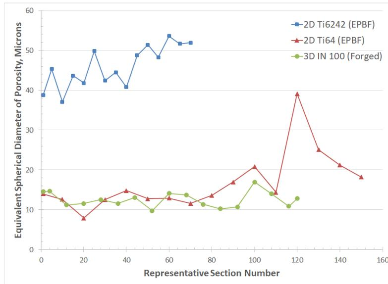
*Figure 11: 2D Slice-to-Slice Variability in Pore Size*
