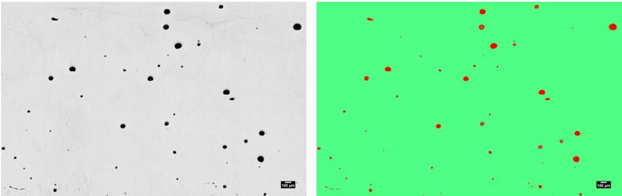
Figure 3: 2D Microstructure and WEKA Segmented Image for Ti6242
