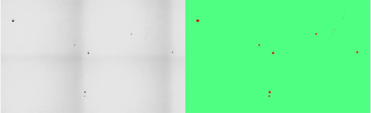
Figure 4: 2D Microstructure and WEKA Segmented Image for Ti64
