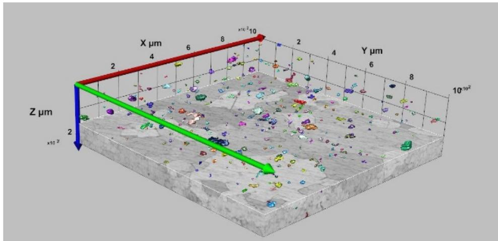
Figure 8: 3D Microstructure and Porosity Distribution for IN 100
