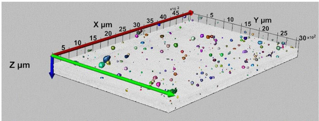
Figure 6: 3D Microstructure and Porosity Distribution for Ti6242
