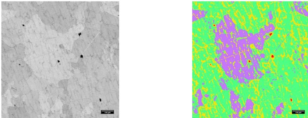
Figure 5: 2D Microstructure and WEKA Segmented Image for IN 100
