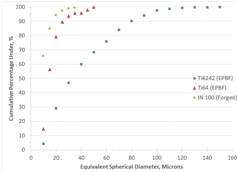
Figure 10: 3D Pore Size Distribution for Ti6242, Ti64, IN 100
