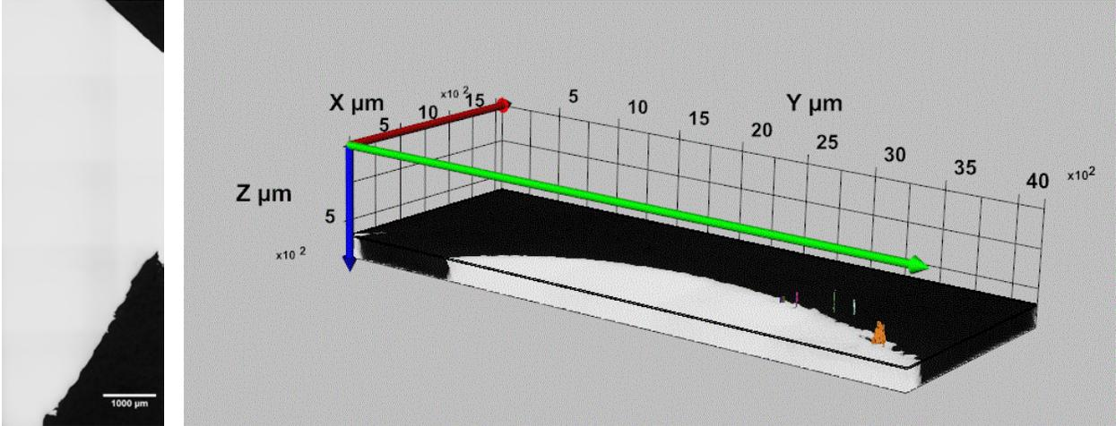
Figure 9: Two (left) Versus 3D (right) Microstructure with Lack of Fusion Defects for IN718
