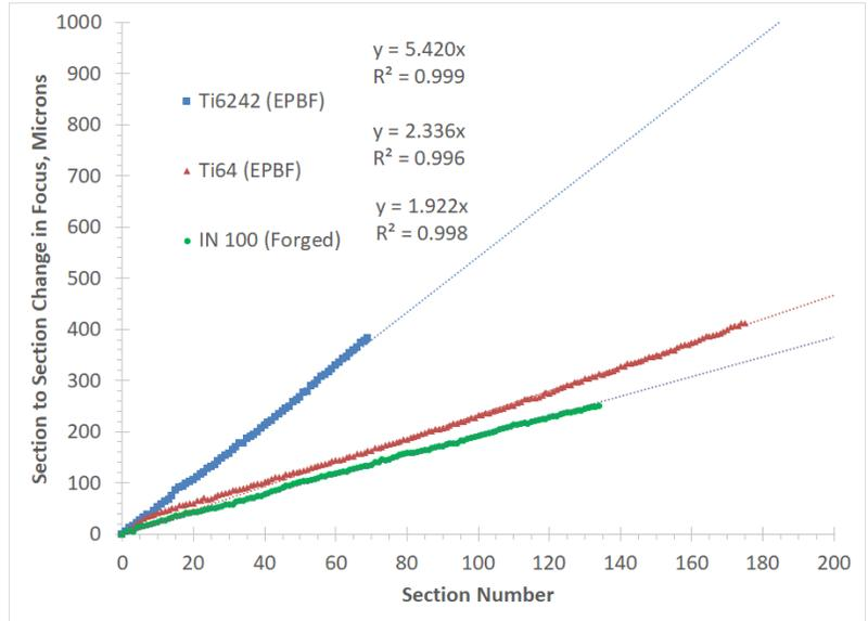
Figure 2: Linear Robo-Met.3D Material Removal Profiles
